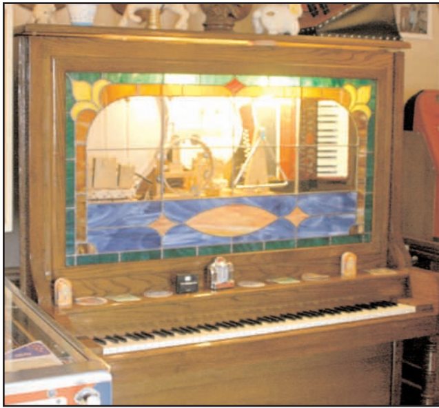
An orchestrion plays music from various instruments when coins are inserted. This one, part of Hockenberger's own collection, includes music made by the piano itself, an accordion, a triangle, drums and bells. Hockenberger is in the business of restoring, repairing and rebuilding instruments like this.
